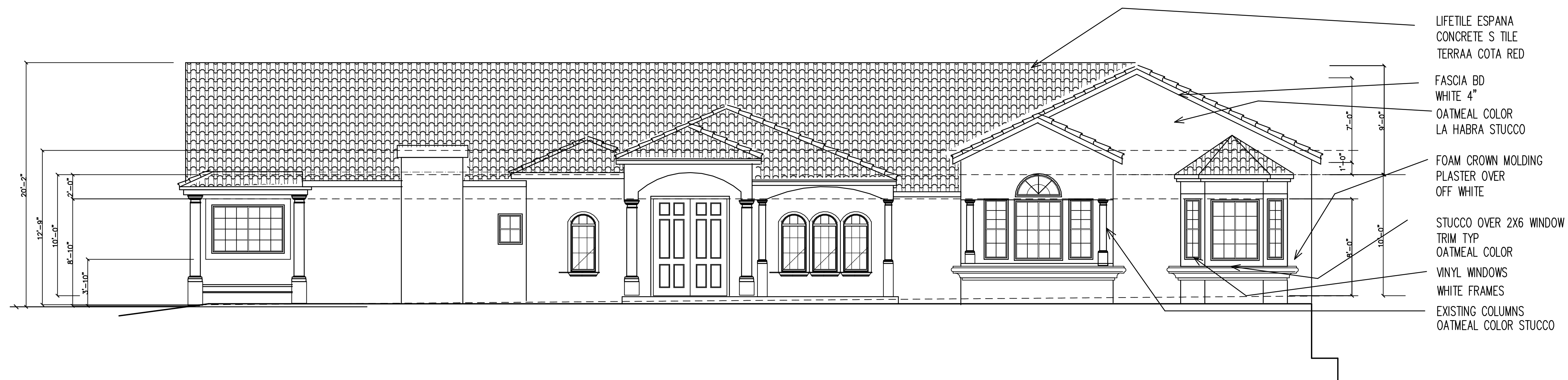
EXISTING EAST ELEVATION
