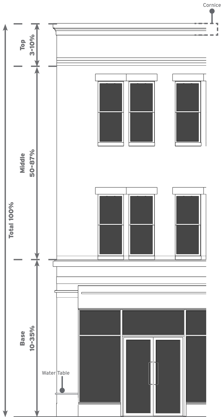
Figure 3-9 - Base Middle and Top Articulation Diagram
