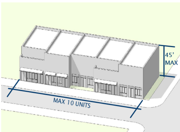
Flex/Loft Building Diagram Example
