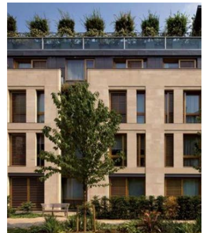
Figure 6-51 - Different Materials Identify Different Façade Planes
