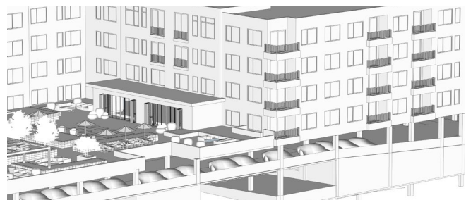
Figure 7-1 - Isometric View of a Podium
